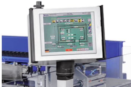
Siemens control system S7 with 12" industrial touch screen
