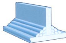
Multiple pass hand welds
