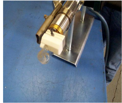
Air outlet, teflon shoe for T-joint welding and emerging PP extrudate
