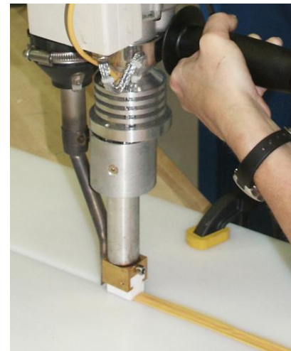
Butt weld performed with Mini extrusion welder on 1/4" thick sheet
